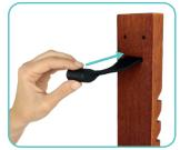
3. Use the included wooden dowel and insert between the strap opening.
